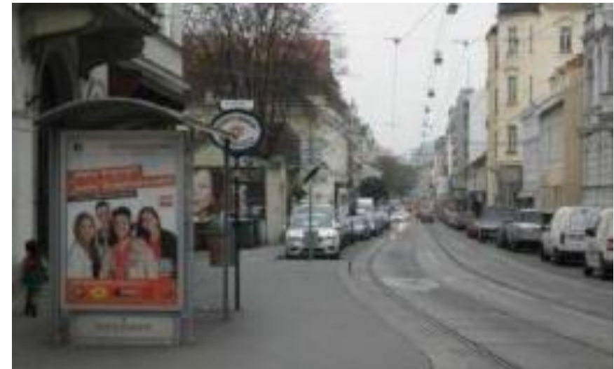
Wien: platform cape prevents overtaking
