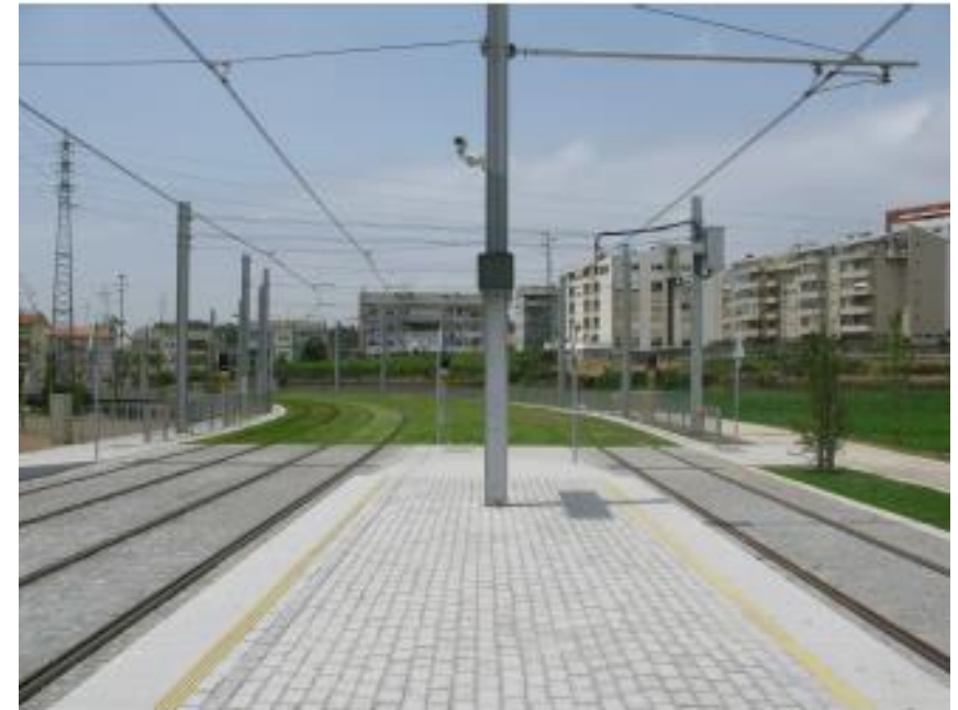
Porto: wider platform, textured surface between rails
