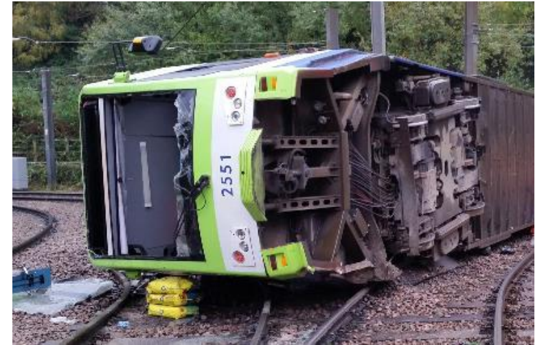
London (Croydon) 2016 Photo: Rail Accident Investigation Branch Tram driver lost awareness and took the corner too fast 7 killed, 19 seriously injured, most other passengers had injuries
