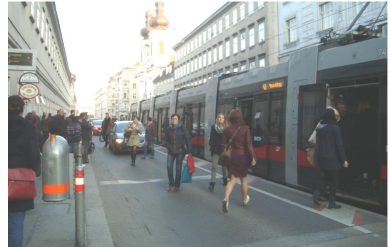
Vienna stop: central track, raised road surface
