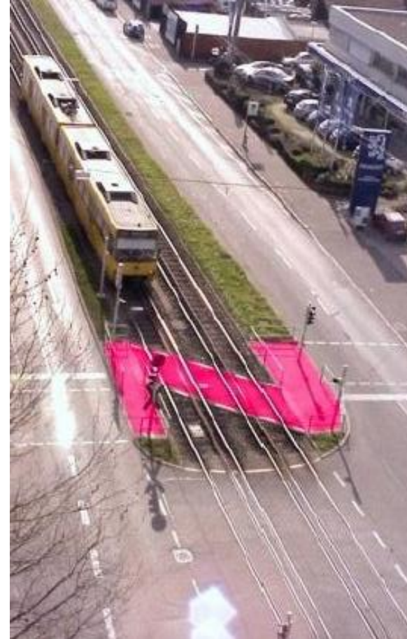
Stuttgart: Z-crossing forces pedestrians to look towards oncoming trams
